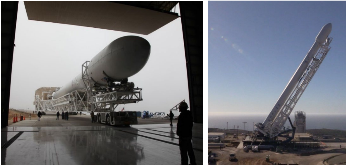
Figure 8-9: Launch vehicle rollout and erection
